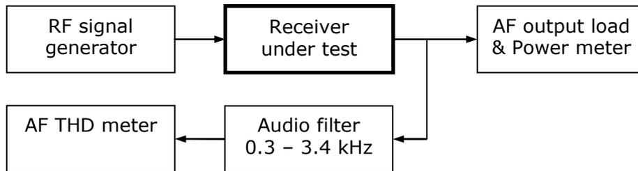
2.2.1.1 Inject a standard RF test signal from the RF signal generator.
