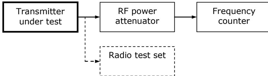
2.3.3.1 Measure the carrier frequency in the absence of modulation.
