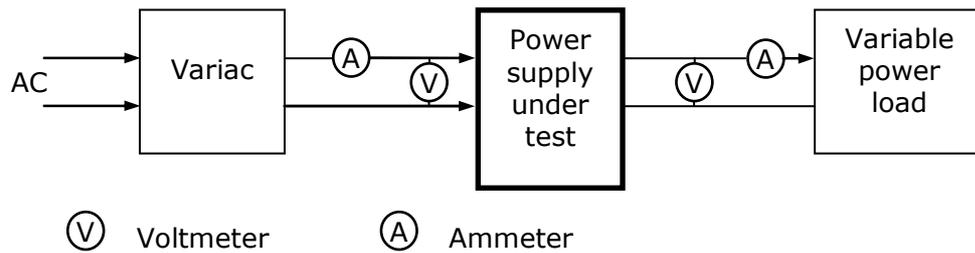
2.4.8.2.1 Adjust the Variac to obtain the nominal input voltage to the power supply/battery charger.
