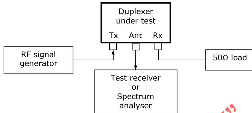
2.4.3.1.3.1 Tune the RF signal generator and the test receiver/spectrum analyser to the in-band transmitting frequency to be measured.
