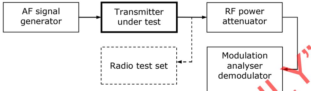
2.3.7.1 Ensure that the maximum deviation is set correctly and according to the manufacturer's procedure.
