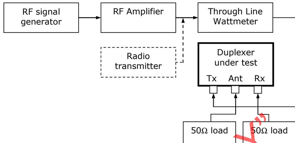
2.4.3.1.5.1 Tune the RF signal generator to the in-band transmitting frequency to be measured.
