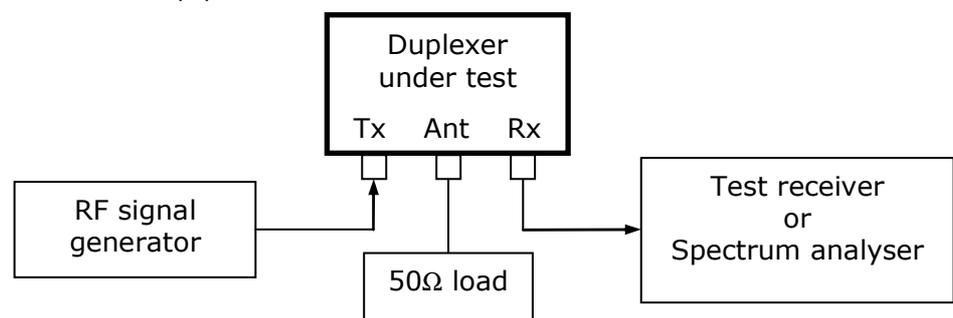
2.4.3.1.4.1 Tune the RF signal generator and the test receiver/spectrum analyser to the in-band transmitting frequency to be measured.
