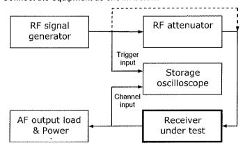
2.2.5.1 Apply a standard RF test signal to the receiver under test.
